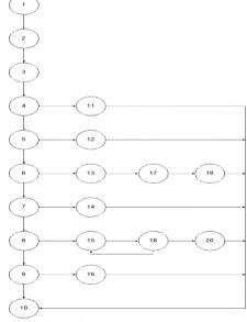
Figure 2. Cyclomatic white box testing
